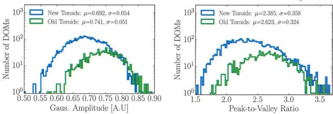
**Figure 7.** Comparison between the AC coupling method used on the DOMs. Left: The Gaussian amplitude fit component,  $N$ . Right: The Peak-to-Valley ratio for the subset of DOMs with different AC coupling.
